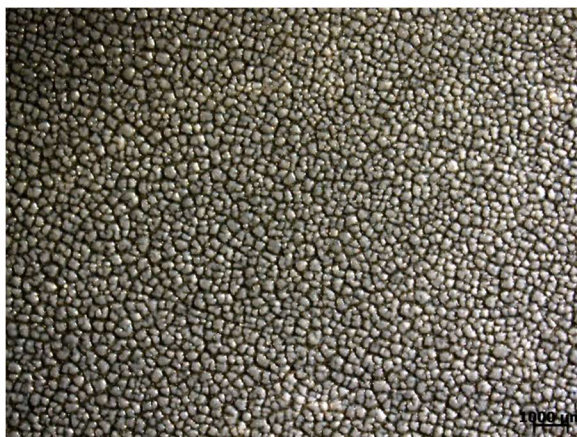
Figure 2 Stereo microscope image of granilla-like effect. The amount of applied material is 60 g solid/m 2 .
