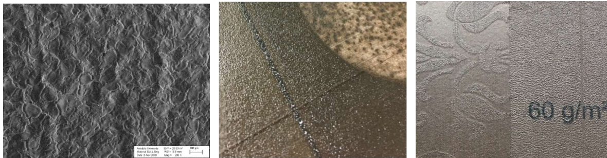
Figure 6 (a) Scanning electron microscopy, (b) and (c) visual photographs of wall tile surfaces with 60 g/m 2 digital ink application.
