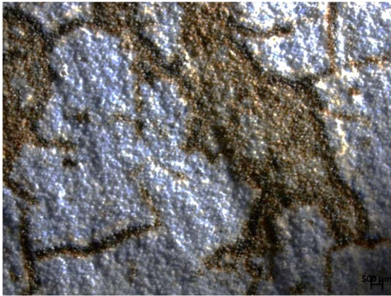
Figure 3 Stereo microscope image of a smooth matt surface showing very fine granular structure. Application amount is 15 g/m 2 .
