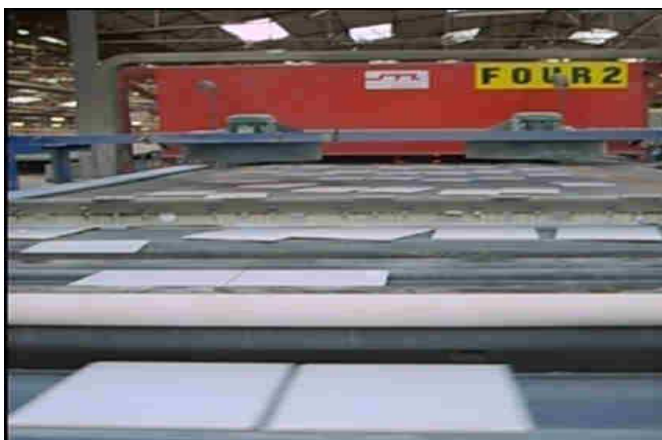
Figure 4. Firing of tiles (200x150 mm) in an industrial kiln
