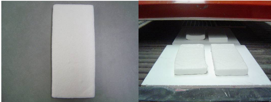
Figure 1. Samples fired at 850°C in a roller kiln
