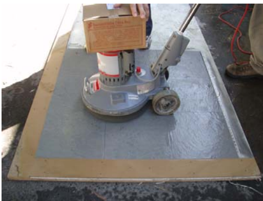
(a) Polishing/buffing machine used to wear tiles
