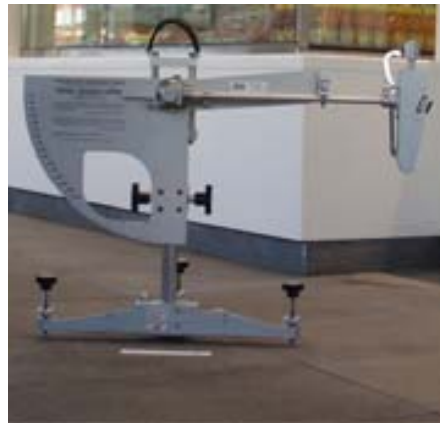
(b) Pendulum slip resistance friction tester
