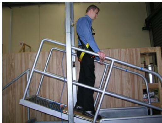
(b) Inclining ramp testing apparatus
