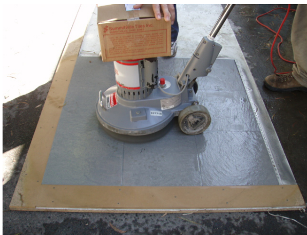
(a) Polishing/buffing machine used to wear tiles
