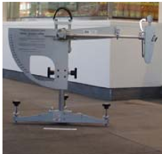
(b) Pendulum slip resistance friction tester
