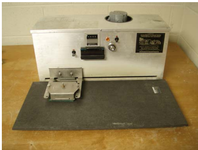
(a) Gardco linear motion washability and wear tester
