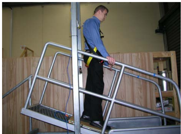
(b) Inclining ramp testing apparatus
