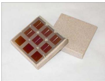
Fig.4a: Small PV cells deposited onto ceramic substrate
